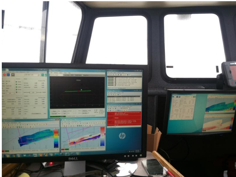
Collecting multibeam data on The Pulse (one of our many vessels)
